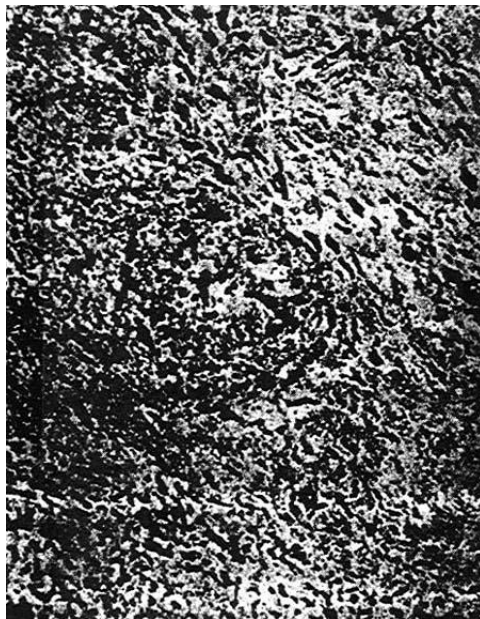
Figure 8. Sample of helical ore in a kaolinite matrix suggesting thermal effects in a clay rich in water with convective movement. Magnification is 100 times.
