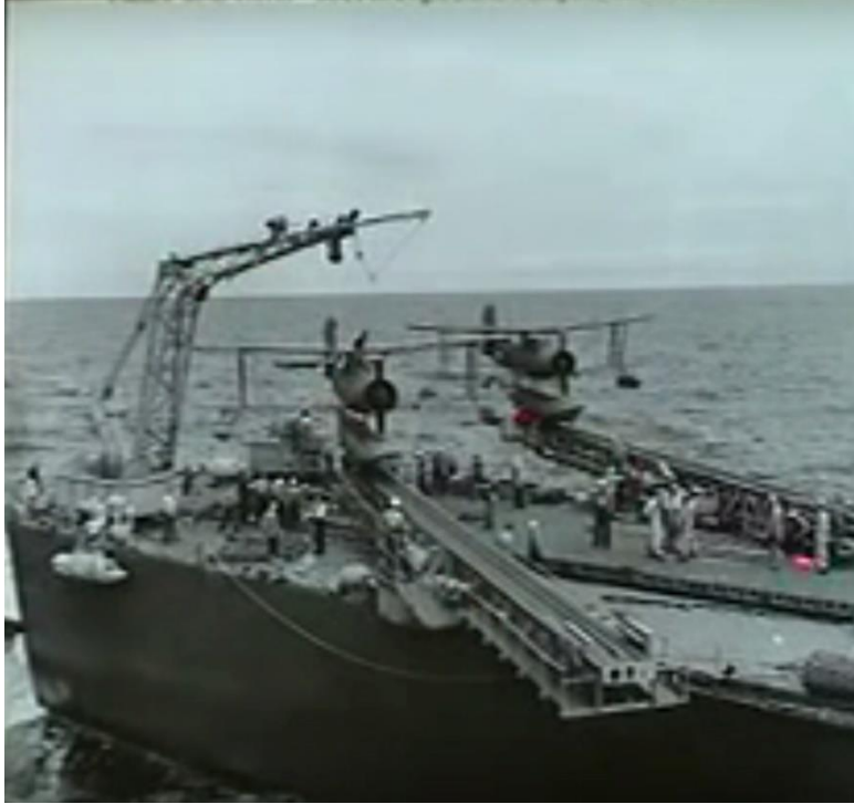
Figure 7. Curtiss SOC “Seagull” scout-observation planes launched from cruisers. Range: 675 miles or 1,086 kms. Pearl Harbor attack was launched from 250 miles out of Pearl Harbor.
