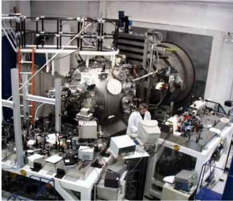
Figure 15. Nike Krypton Fluoride KrF laser chamber at the Naval National Laboratory, NRL.
