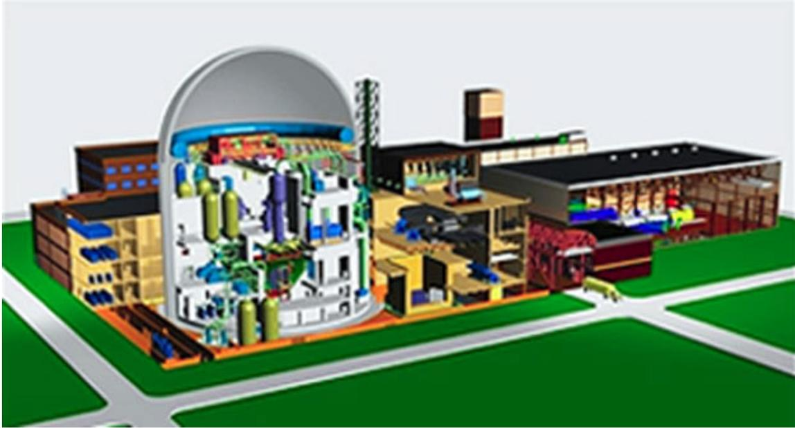
Figure 11. Cutout diagram showing a Candu 9 plant setup.
