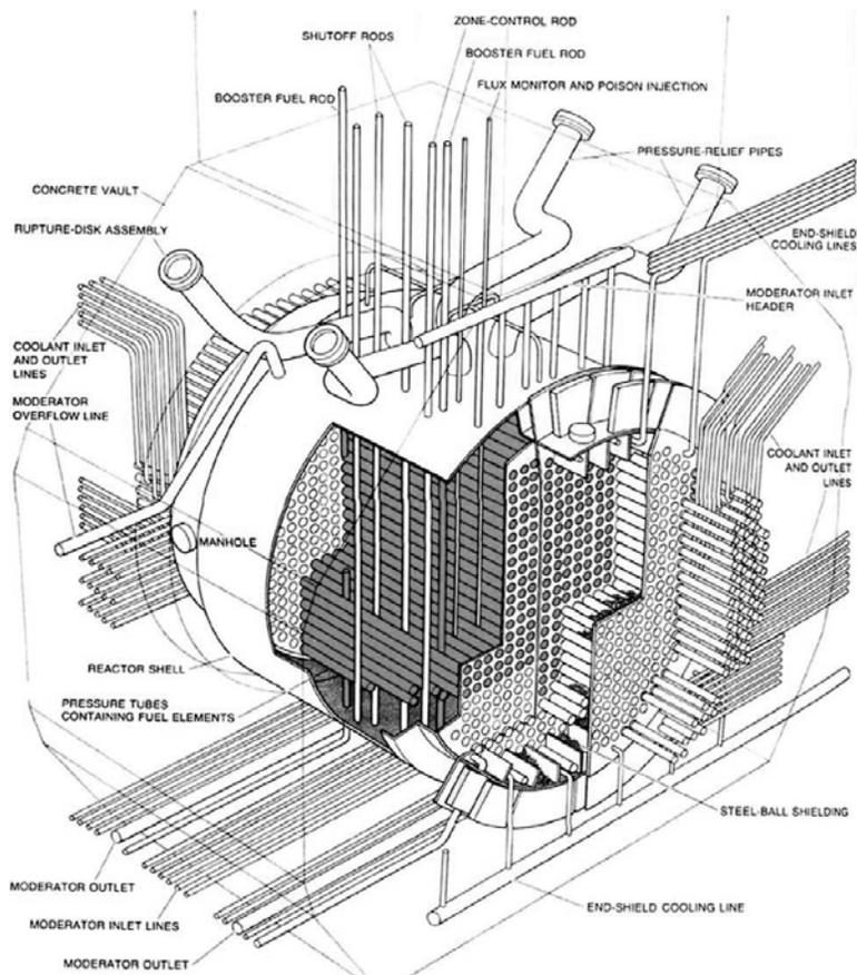
Figure 5. Horizontal calandria of HWR showing its components.
