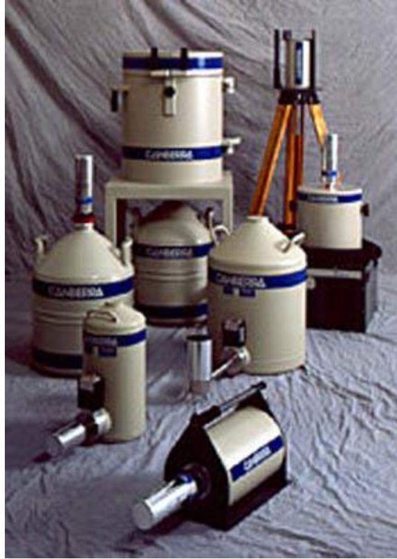
Figure 14. Germanium detectors and their background radiation shields and cooling cryostats.
