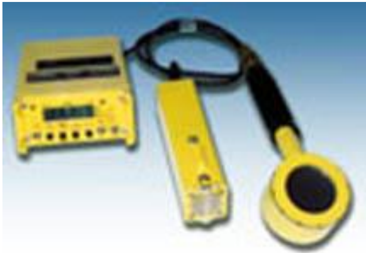
Figure 24. Survey meter and smart probes for beta, alpha and x-ray and gamma radiation.
