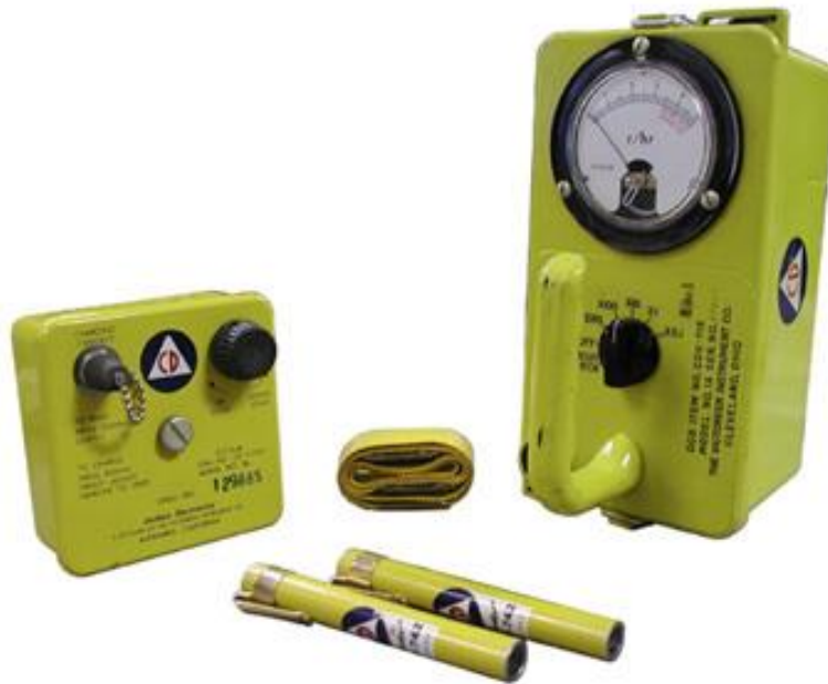
Figure 5. Cold war period fallout shelter survey meter, ionization chambers and their charger.
