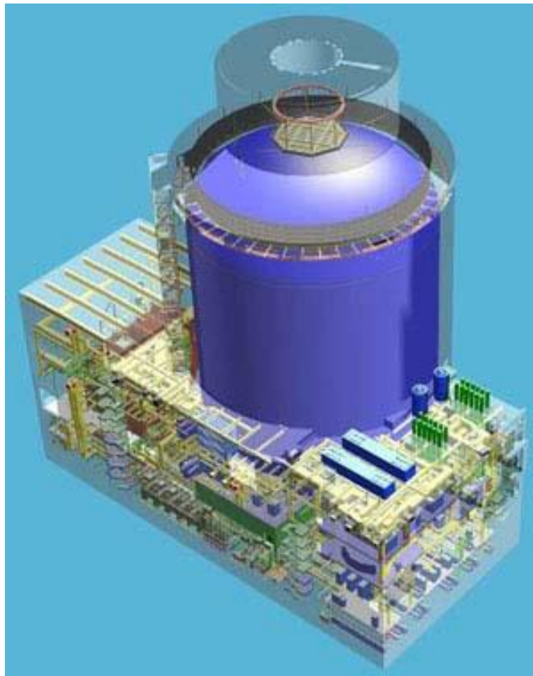
Figure 2. Cutout of the AP1000 showing its chimney concrete containment structure surrounding its steel shell containment.
