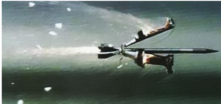
Figure 5. The sabot detaching from a depleted uranium projectile.
