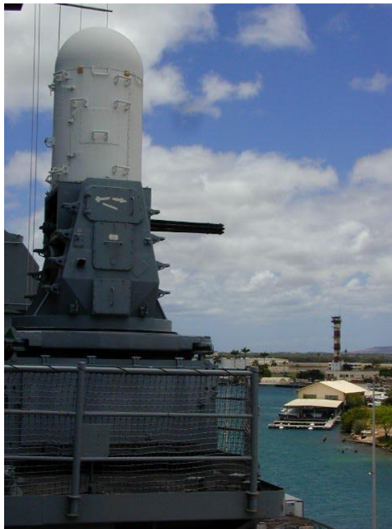
Figure 9. Depleted Uranium Gatling gun radar assembly on the USS Missouri, Pearl Harbor, Hawaii, for interception of oncoming missiles and attacking fast boats. Photo: M. Ragheb.
