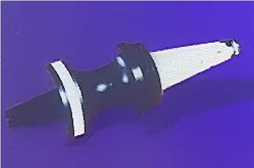
Figure 7. Carbon-fiber composite sabot for a depleted uranium projectile.
