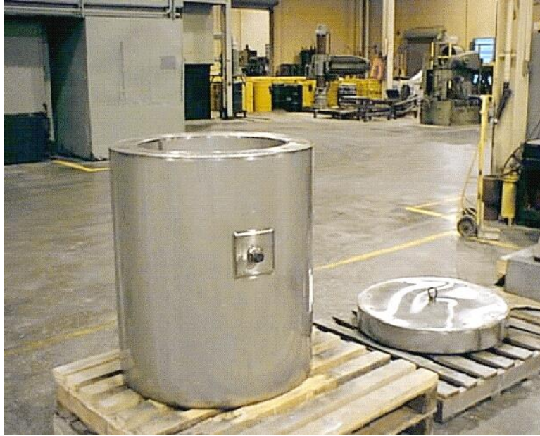
Figure 10. Depleted Uranium used as a DUCRETE concrete aggregate in a radiation shielding cask.
