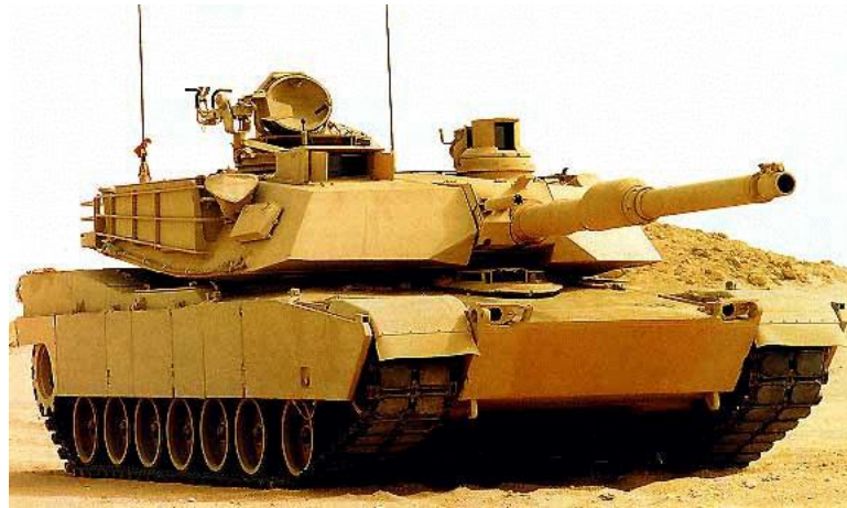
Figure 1. The USA Abrams M1A1 tank uses depleted uranium and boron ceramic armor plates and fires depleted uranium munitions. High carbon steel and composite boron ceramic act as shield against radiation. Source: USA Army.
