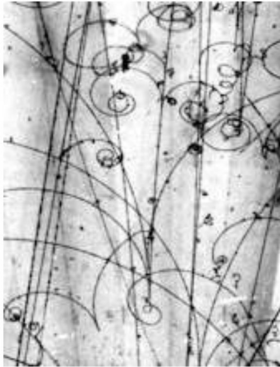
Figure 2. Bubble chamber tracks of electron-positrons pairs diverted in opposite directions along a magnetic field perpendicular to the page.
